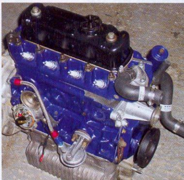
19. The finished assembled engine ready for installation. Note the flow-efficient block to filter head transfer pipe. I really don't like the standard set-up — it's very restrictive.
