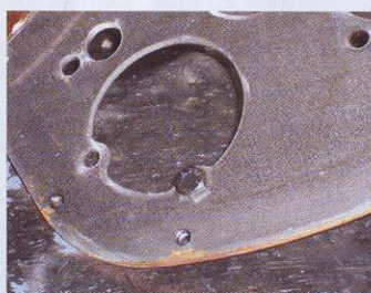
7. When changing to a duplex (twin row chain) cam drive set-up — advisable where performance cams and stronger valve springs are used — it's necessary to alter a couple of things. First is the front plate to main cap retaining bolts. As standard where simplex (single row chain) cam drives are fitted, these are standard-type bolts.
