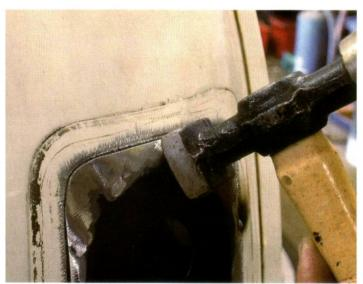
9. If any areas are slightly proud then use a body hammer to make any adjustments. If you have not removed enough metal from the panels then you'll have to grind through the welds and start again.
