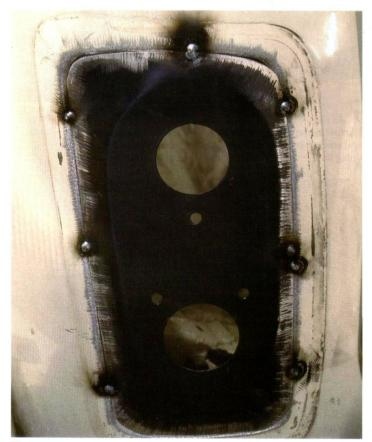
7. Once you are happy with the shape and profile of the panel, clean up the edges to remove the protective layer of paint and tack them into position. You only need a few tacks at this stage, just enough to hold it in place whilst you make any last minute adjustments.
