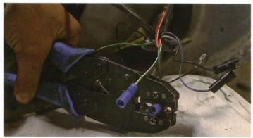
6. The old MkI lights use bullet style connectors, so get half a dozen female bullet terminals and simply crimp them onto the existing wires. Ensure that the terminals are crimped securely, otherwise the lights may fail.
