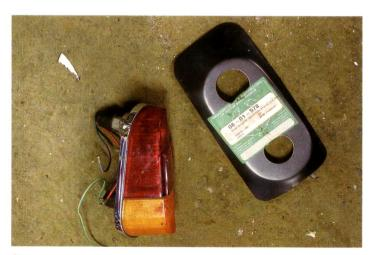
2. New and second-hand lights are available; when buying second-hand units ensure that they still have the wiring intact and that the lenses are in good condition. As mentioned, the Hadrian Panels conversion plates can be sourced from most good Mini specialists.
