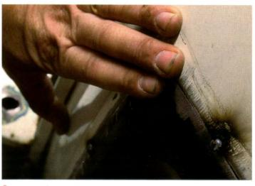
8. The best way to check that the panels fit well is to use your hand (allow the welds to cool first!) and feel the transition between the new panel and the rear of the car. This should be as smooth as possible.
