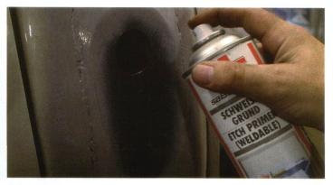
4. We applied a coat of etch primer first as we are still a long way off being ready for filler and paint. Use a good quality filler to cover the weld line and, providing you took your time and did it correctly, you should only require a very thin layer of it.
