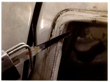
4. You will need to remove the paint from around the old light aperture. I prefer to use an air saw with the blade just scratching the paint off. You can use a sanding disc in a grinder or similar, but take care not to remove too much metal at the same time!
