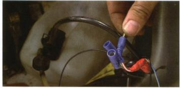
7. The colour code is the same on the early and late Minis so simply connect the corresponding wires together. You'll have one spare wire left over on the old loom, as the new lights do not have a reverse fitted.
