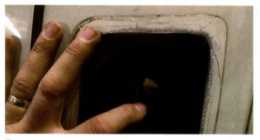
5. Like most things, the plate will need a little bit of trimming to get it to fit properly. You may also need to shape it slightly to follow the contours of your car. Mark the panel where you need to trim it.
