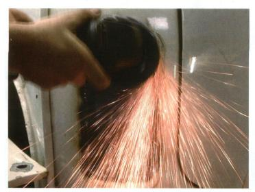
2. Once the panel has cooled down, dress back the weld using a sanding pad in a grinder. Remember to wear eye protection and, as when welding, move around to prevent unwanted heat build up.
