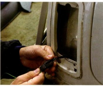
First job is to remove the old light units. This is done by undoing the securing nuts from inside the boot and then disconnecting the electrical connection. We sold our old units on eBay to recoup some of the cost of the conversion.
