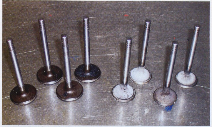
4. Here are the old valves from test head one. They are in remarkably good condition so we'll re-use them. The light grey deposit on the exhaust valves is synonymous with unleaded fuel use.
