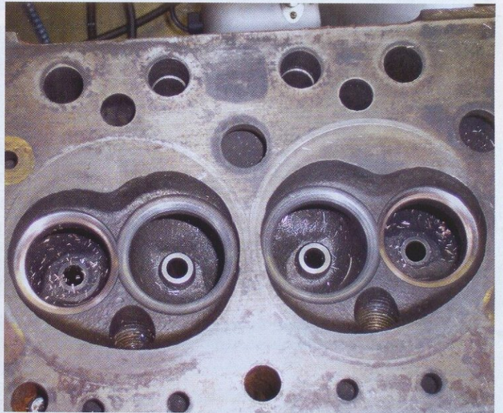
14. Here are the new three-angle seats recessed down into the chamber to sink the exhaust valves far enough down to give clearance to the block when the exhaust valve is at full lift. The inlets are not cut down quite as far as this is unnecessary. You can clearly see the colour of the beryllium-copper exhaust valve seat inserts, which were fitted at the factory for unleaded fuel compatibility.
