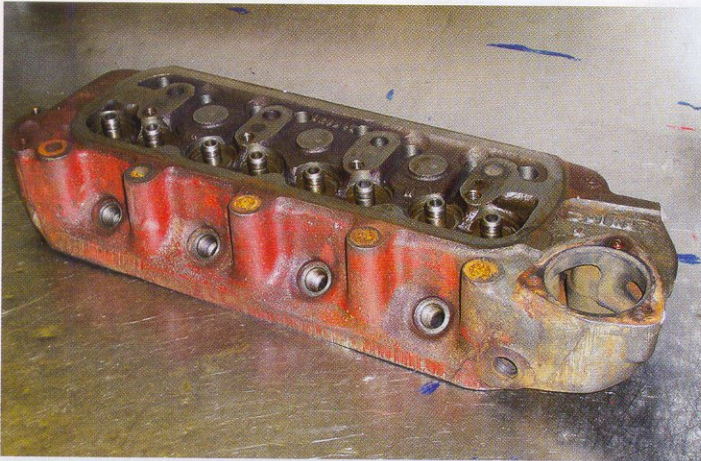
1. Test head number one: a standard A-plus I275, easily identified as such by the sculptured upper surface around the thermostat and heater tap areas. This is a Metro head but is the same as just about all other A-plus castings — the only difference from the MG and Van Den Plas Metro heads is the larger size inlet valve (35.7 mm as opposed to 33.3 mm), which can only be identified by having the head off the block and measuring it. This particular head had exhaust seat inserts already fitted.
