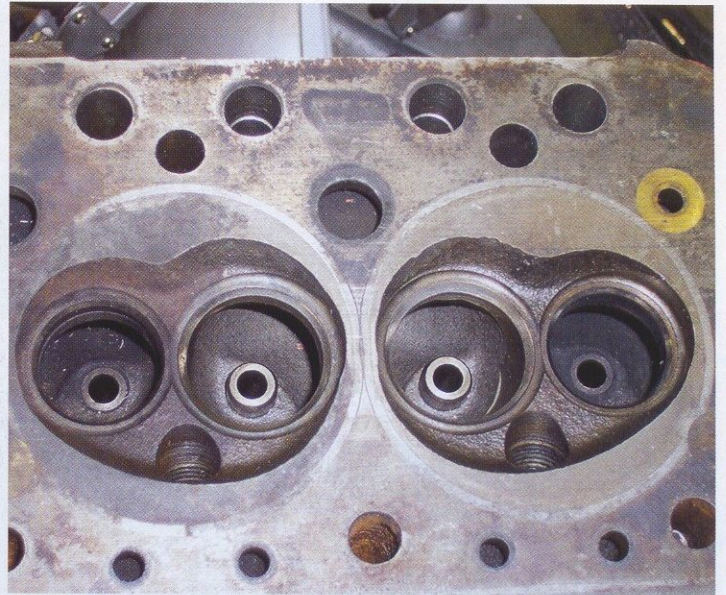
13. Here are the standard seats prior to re-cutting. The seat outer edges are at the same level as the chamber roof valve reliefs — no top-cut angle and no under-cut angle, just wide 45-degree angles.
