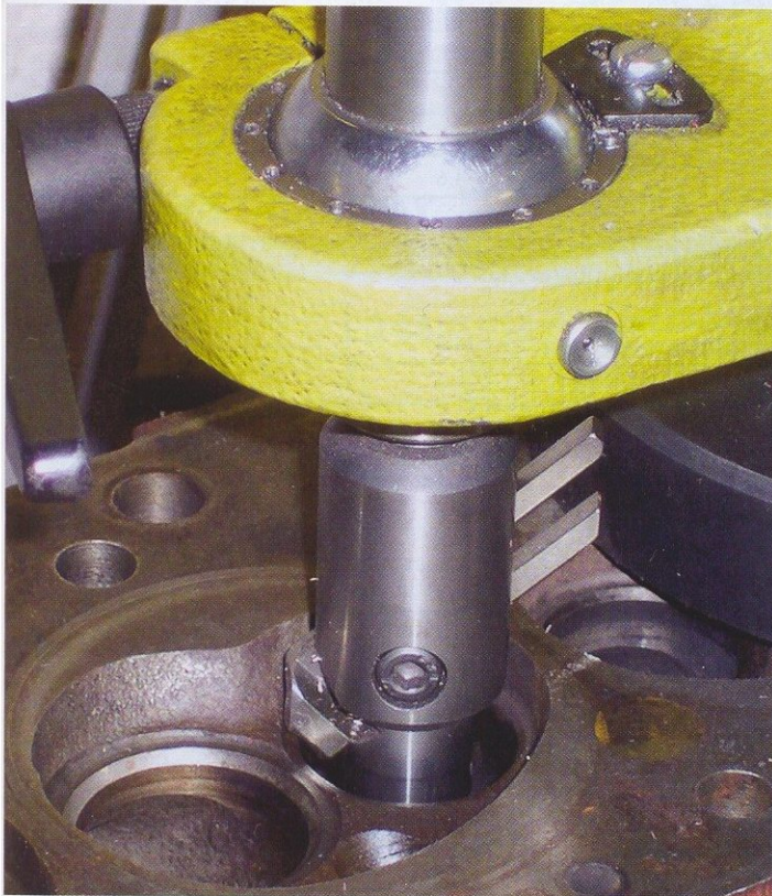
12. This is my seat cutter — a MIRA. It uses a rotating pilot that locates in the valve guide, and multi-angle tools to cut three angles at the same time — top-cut above the seat, the seat and then an under-cut below the seat. Messing with these angles gives interesting effects. Here I'm using a fairly standard 30-degree top-cut, 45-degree seat and 60 degree under-cut. Seat width is 0.05 inch.
