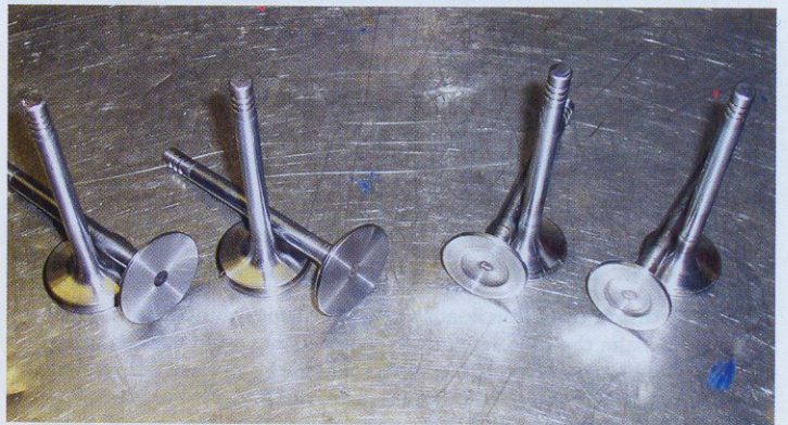
6. The result of a few minutes' work with the drill and abrasive tape — nice shiny valves.
