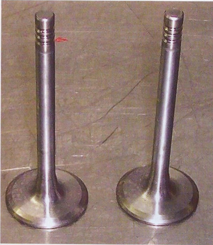
11. The inlet valve seats were also re-faced and then a 30-degree back cut applied to reduce the seat width as per the exhaust valves. This gives better airflow, particularly when the valve seat width is less than the head seat width.
