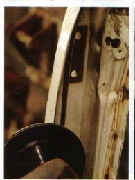
Our car required new A-panels anyway, so these were removed along with our rotten front vings. We'd already cut away the majority of the rusty A-panels and just had to use a grinder to remove the lip at the rear edge of the panel where it wraps around the hinge panel. It's also necessary to remove the door and the old hinges.
